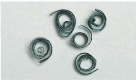
Very tight chip winding or showing bluish shades: feed too high
