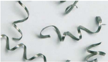
Moderate chip winding: correct cutting conditions
