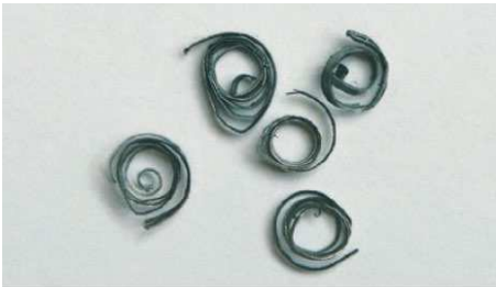
Very tight chip winding or showing bluish shades: feed too high
