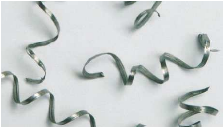
Moderate chip winding: correct cutting conditions
