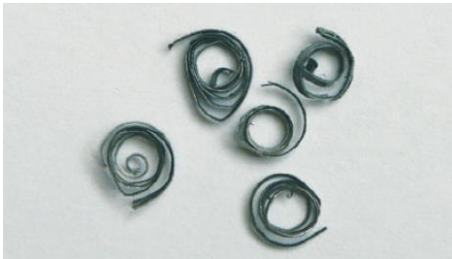
Very tight coiling or with bluish tones: feed rate too high
