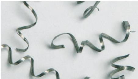
Moderate coiling; correct cutting conditions
