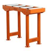
Fixed tables available in lengths of 1 metre and 2 metres - Height-adjustable legs: 800 to 1000 mm - Maximum load: up to 1400 kg depending on model - Ball bearing roller axles for smooth sliding and increased durability - Floor mounting for perfect stability.
